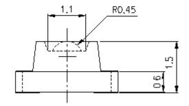
For reflow soldering (propose)
