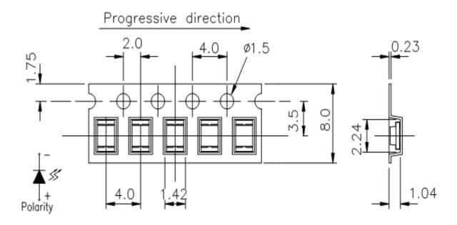
**Note:** The tolerances unless mentioned is  $\pm 0.1$ mm, Unit = mm
