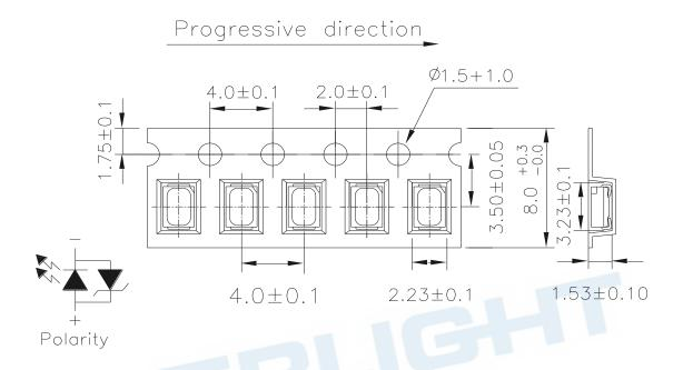
**Note:** Tolerances unless dimension are  $\pm 0.1$ mm, unit = mm.
