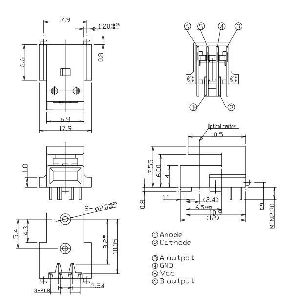
Dimensions are in millimeters.
